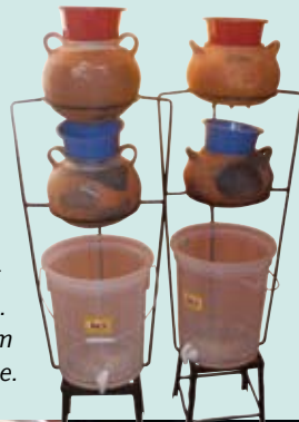
(Right) Water drips through a series of containers that hold a naturally purifying compound in the bottom.
