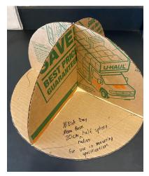
Fig 2. Sample internal measurement tool. The safe zone tester was created by Julian Peña, Lead Judge with the San Jose State University MESA Center.
