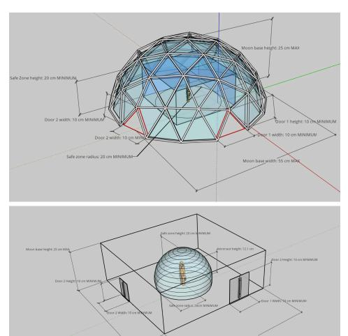
Fig 1. Clearances and dimensional specifications for space to fit the structure. These diagrams are a representation to show the MINIMUM interior dimensions of structures for the safe zone and MAXIMUM exterior dimensions of the Moon Base. Please note that the interior and exterior shape and placement of the openings of the Moon Base is to be determined by teams within the minimum and maximum requirements.
