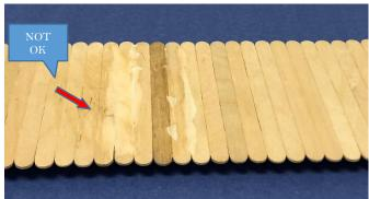
Glue is visible on areas other than the joints and the remains of wax paper left on the roadway are considered coating. Easy way to fix this is to sand off the excess glue or wax paper.
