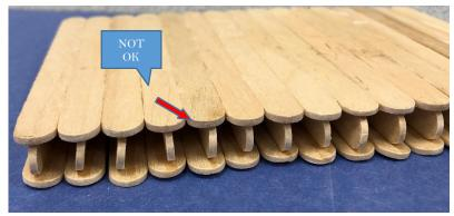
I-Beams are illegal in the bridge's structure.
