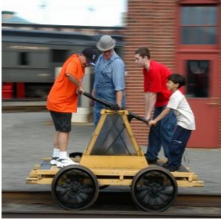
Figure 1. A handcar, a simple machine that operates on the principle of the lever.
