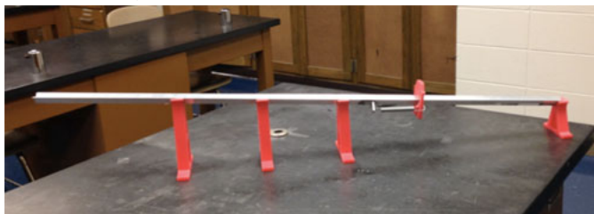
Figure 1. A homemade glider launcher using 3D-printed support legs and launch block.
