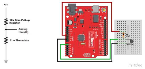
Write an equation for the voltage across the Thermistor. Let's call it V<sub>therm</sub>.
